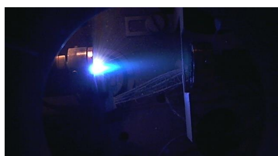
Plasma plume during the laser based deposition of tungsten.
