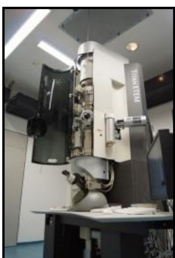
Titan 80-300 environmental atomic-resolution scanning / transmission electron microscope.
