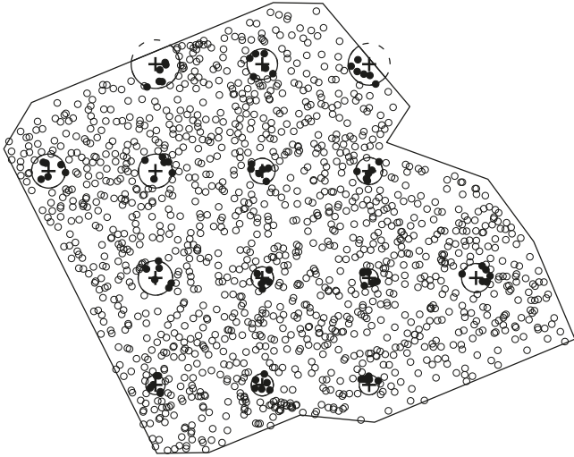
Fig. 3. Positions of trees in a forest stand (STIPSI 28). Fourteen six-tree sample plots (large circles) are placed in a regular 50 m grid with a random start. Measured trees are shown as solid circles.
