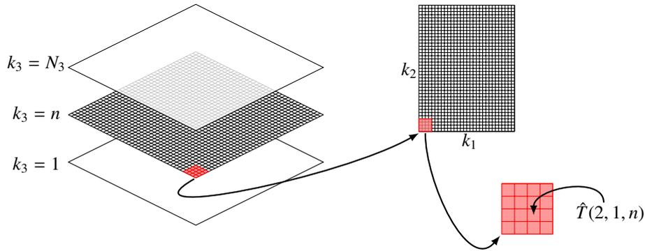
Figure 3.2: Data structure of temperature field within the global GPU memory. Other data arrays are structured in a similar way. This arrangement allows easy pointer arithmetic to iterate through the data. Moreover batched fast Fourier transformations are possible.
