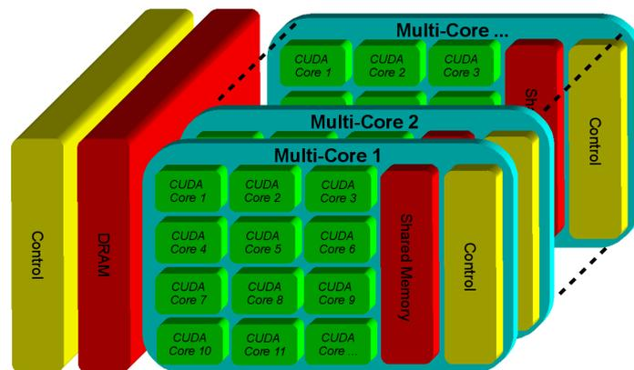
Figure 3.1: Layout of a CUDA GPU. Each GPU consists of multiple Multi-Cores. All Multi-Cores have access to the global memory of the GPU. A Multi-Core has many CUDA-Cores and all of them have access to the shared memory. The CUDA-Cores themselves have several registers and some local memory.
