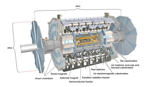
Figure 1.1: Schematic view of the ATLAS detector [1].
