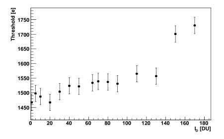
Figure 5.12: Minimum threshold versus discriminator current  $I_D$  without sensor.
