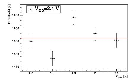
Figure 5.1: Dependency of the minimum threshold on the analogue voltage  $V_{DDA}$  without sensor.
