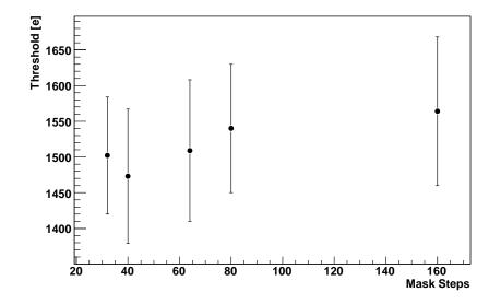
Figure 5.16: Dependency of the minimum threshold on mask steps without sensor.
