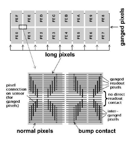
Figure 2.3: Schematic drawing of the different pixel types [4].
