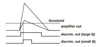
Figure 2.5: Amplifier output and discriminator response for different feedback currents [4].
