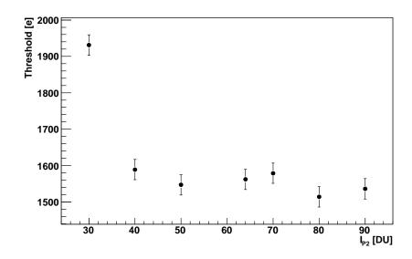
Figure 5.10: Dependency of the minimum threshold on the amplifier current  $I_{P2}$  without sensor.
