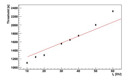
Figure 5.6: Dependency of the minimum threshold on the feedback current  $I_F$  without sensor.
