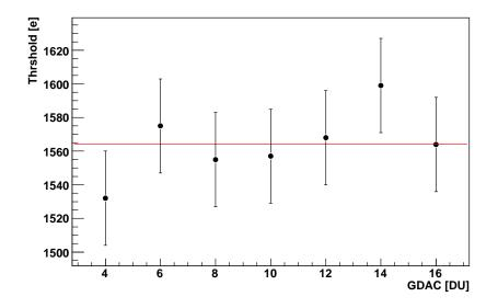
Figure 5.14: Dependency of the minimum threshold on GDAC without sensor.
