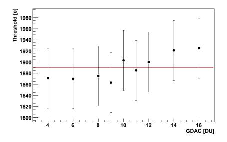
Figure 5.15: Dependency of the minimum threshold on GDAC with sensor.
