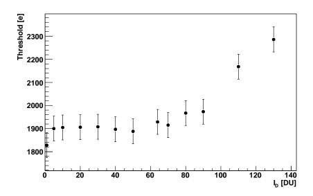
Figure 5.13: Minimum threshold versus discriminator current  $I_D$  with sensor.
