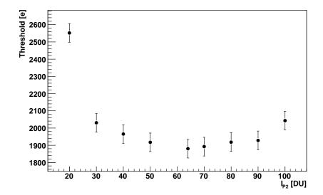
Figure 5.11: Dependency of the minimum threshold on the amplifier current  $I_{P2}$  with sensor.
