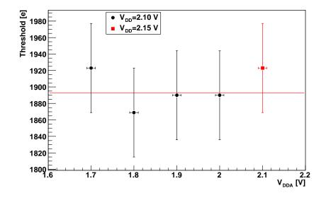
Figure 5.3: Dependency of the minimum threshold on the analogue voltage  $V_{DDA}$  with sensor.
