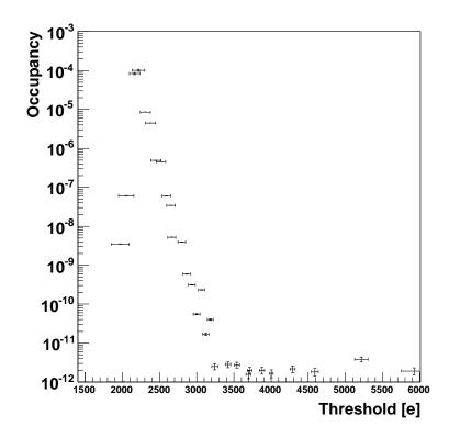
Figure 4.1: Occupancy versus threshold from the hitbus measurement with sensor.
