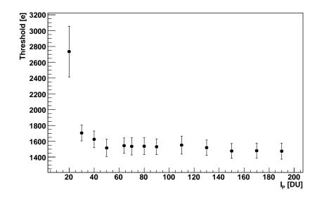
Figure 5.8: Dependency of the minimum threshold on the preamplifier current  $I_P$  without sensor.
