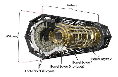
Figure 2.1: A schematic view of the pixel detector consisting of barrel and endcap layers [3].
