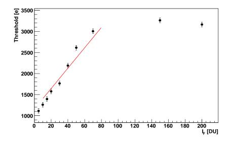
Figure 5.7: Dependency of the minimum threshold on the feedback current  $I_F$  with sensor.
