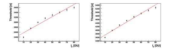
Figure 5.5: Dependency of the standard threshold on the feedback current  $I_F$  without sensor (left) and with sensor (right).
