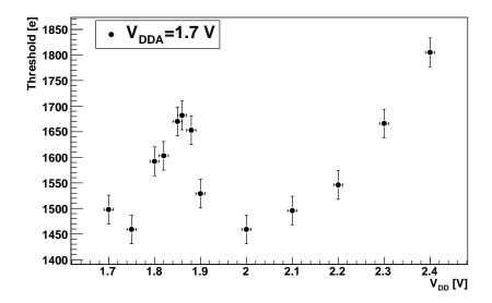
Figure 5.2: Dependency of the minimum threshold on the digital voltage  $V_{DD}$  without sensor.
