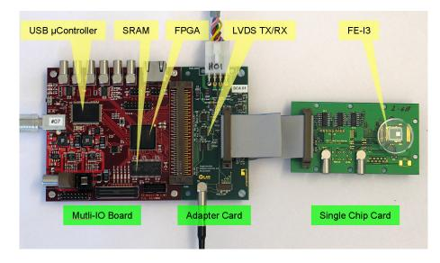
Figure 3.1: UBSPix board with single chip card [9].
