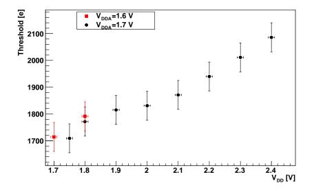
Figure 5.4: Dependency of the minimum threshold on the digital voltage  $V_{DD}$  with sensor.
