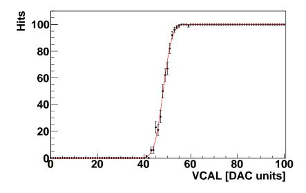
Figure 3.2: Hits versus VCal, which corresponds to the injected charge.
