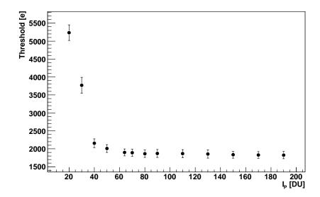
Figure 5.9: Dependency of the minimum threshold on the preamplifier current  ${\cal I}_P$  with sensor.
