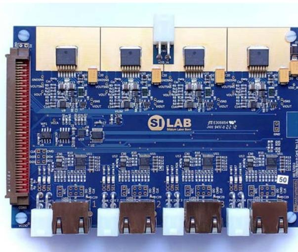
Figure 3.2: The burn-in adapter card, supporting connection of up to four FE-I4 chips simultaneously.
