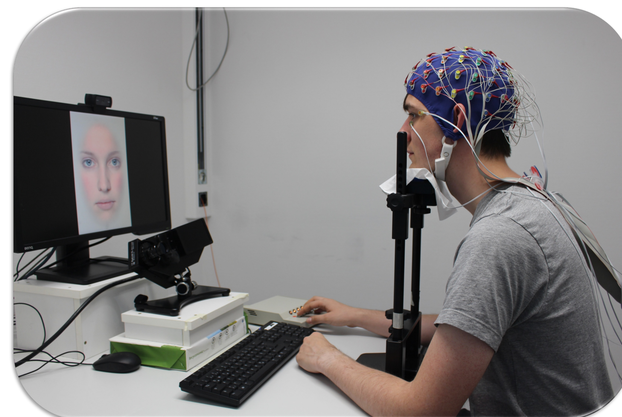
Fig. 2: Exemplary experimental setup with EEG and eye-tracking recording.
