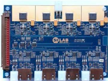
*Figure 4.1.:* The burn-in adapter card for the MultiIO board.
