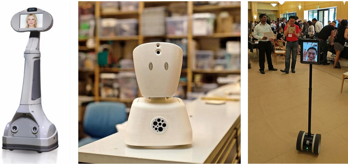
Figure 1: Selection of telepresence robots. Left: VGo [6], image source: Dmitry Suvorov, Wikimedia Commons, CC BY-SA 4.0. Center: AV1 [20], image source: Mats Hartvig Abrahamsen, Wikimedia Commons, CC BY-SA 4.0. Right: Double, image source: Steve Jurvetson, CC BY 2.0.
