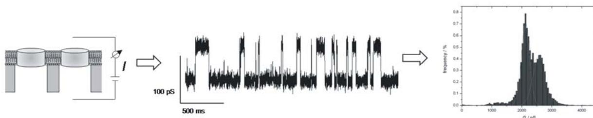
**Figure 1.** Schematic diagram of the setup of a single channel recording with subsequent evaluation.
