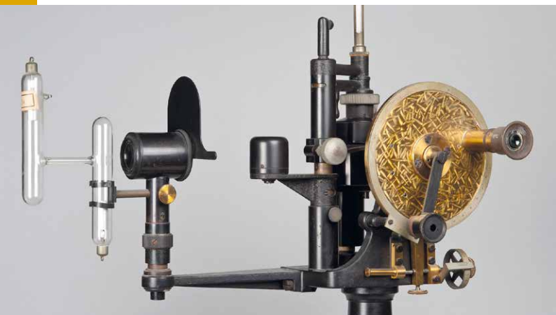
Pulfrich refractometer , 1895. photo: Stephan Eckardt
