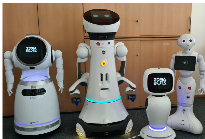
Fig. 1. Robots with different appearances and sensors. From left to right: CruzR [6], Car-O-Bot 4 [7], James [8], and Pepper [9].
